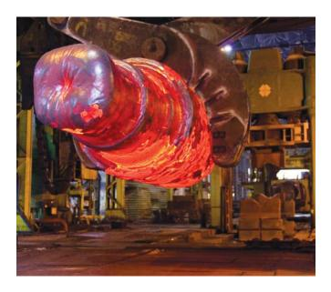
The research team monitored the expansions and contractions of the metal, through cooling after casting and through heat treatment, to test for strength and fatigue resistance. The team used computer simulations to help achieve the extremely high quality standards required. These simulations modelled the extreme loadings likely to occur in operational conditions.
